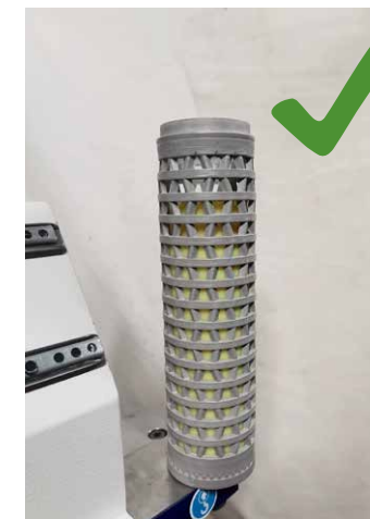
Inspection of the bobbin passing through the dyeing machine. Acceptable.
