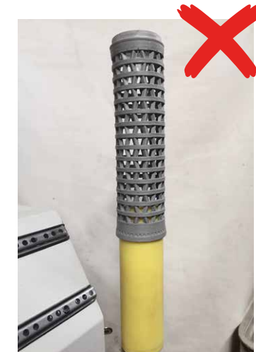
Inspection of the bobbin passing through the dyeing machine. Unsuitable.
